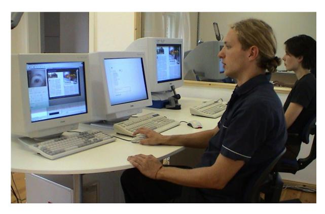
Eye tracking solutions were also utilized for studies conducted on desktop computers. our labs, we examined the online reading behavior of participants using SMI eye tracking technology. Eye movements and gaze directions were monitored semi-automatically with a video camera.
