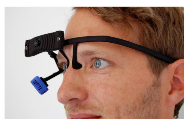
An advanced stage of mobile eye tracking is represented by the Head-Mounted Pupil Labs Eye Tracker, which incorporates built-in webcams. The initial evolution from laboratory settings was webcam eye tracking using a camera installed on a PC, allowing for cost-effective and rapid measurement of gaze patterns.
